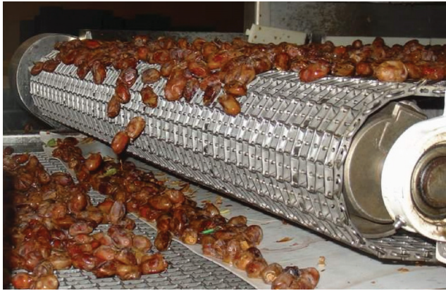
Plate 8.2 Chain conveyor moving Khalal dates after sorting. Reproduced with permission of S.M. Aleid.
