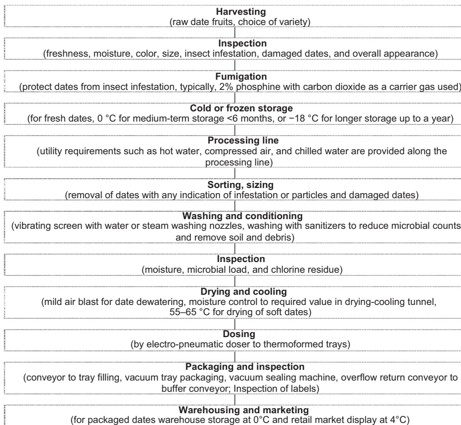
Figure 8.1 Flow diagram for the commercial date processing.
