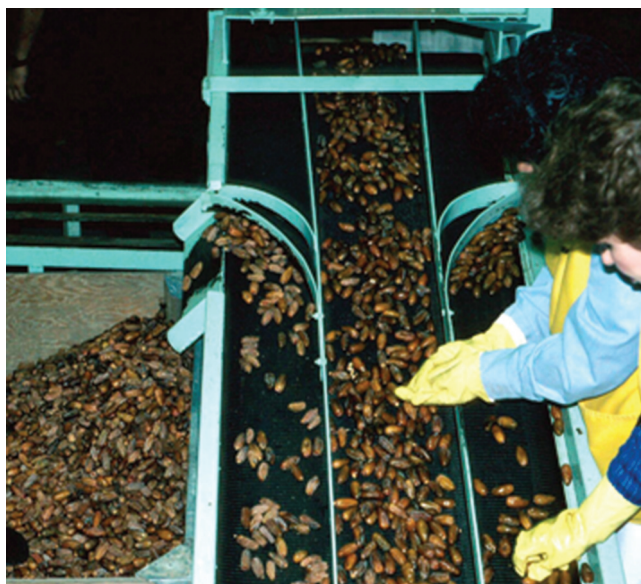
Figure 5.5 Manual sorting of dates on a conveyer belt. Courtesy A.A. Kader.
