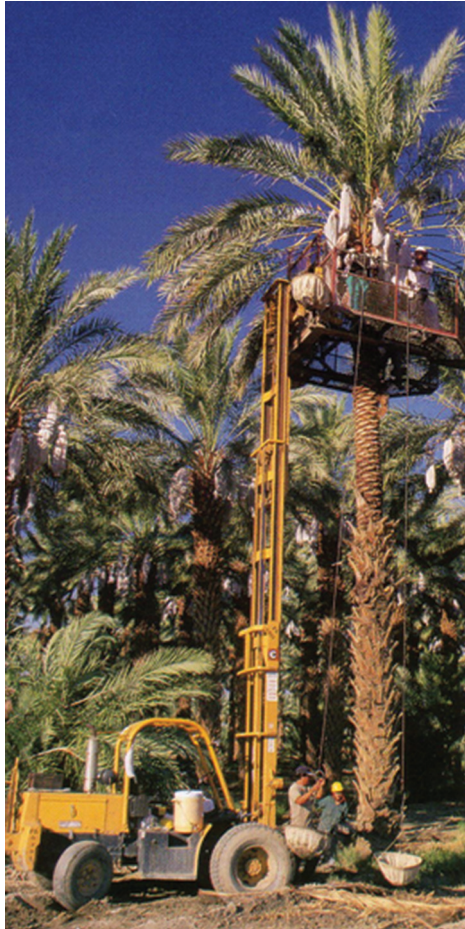
Figure 5.2 Hydraulic-crane built on a truck used by the picker to reach the top of the tree. Reproduced with permission of Davis Karp.
