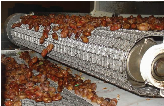
Figure 8.2 Chain conveyor moving Khalal dates after sorting. Reproduced with permission of S.M. Aleid. (For a color version of this figure, please see the color plate section).
